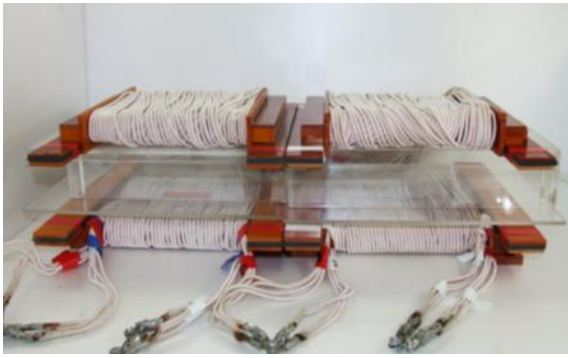
(a) Photograph of module configuration transformer.
