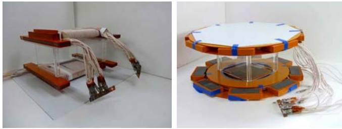
(a)H-shaped Transformer's outline. (b)Circular Transformer's outline.
