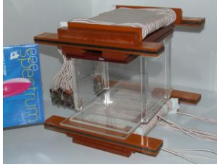
Figure 6. Photograph of transformer.
