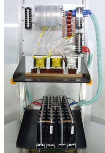
Fig. 7. Current-doubler rectifier with LC filter and EDLCs.
