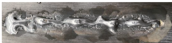
Fig.2 Bead appearance without magnetic field
