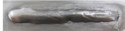
(b) Conditions for suppressing bead-meandering while maintaining bead width. (AC right-left oscillation, B_{RMS} = 0.5 mT, f = 100 Hz)
