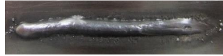
(a) Conditions that suppressed bead-meandering the most. (AC front-back oscillation, B_{RMS} = 1.0 mT, f = 100 Hz)
