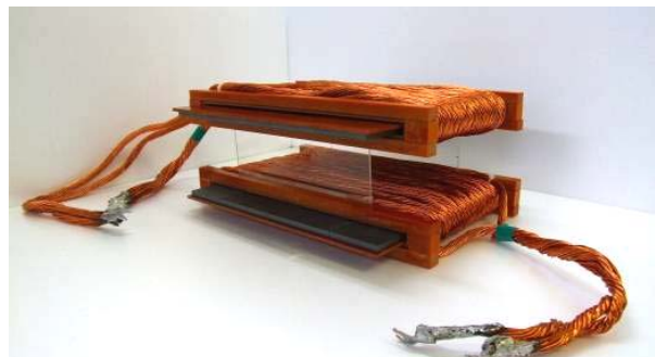
Fig. 6. Photograph of 1.5 kW transformer
